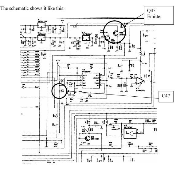
12 VDC can be taken from any point where it is convenient and the ground can be connected to any convenient point that is connected to the chassis ground. On the 706, the Q45 Emitter (shown above) turns out to be a convenient place to tap for 12 VDC power and there are a number of caps in the vicinity with one side connected to chassis ground.
