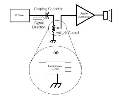
In the IC706, this is at capacitor C47 as shown below.
